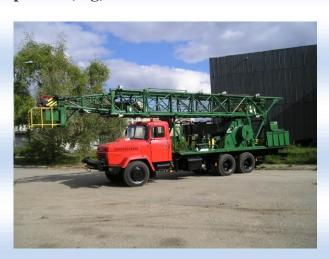
single-drum with chain drive, friction clutch's to engage drum
