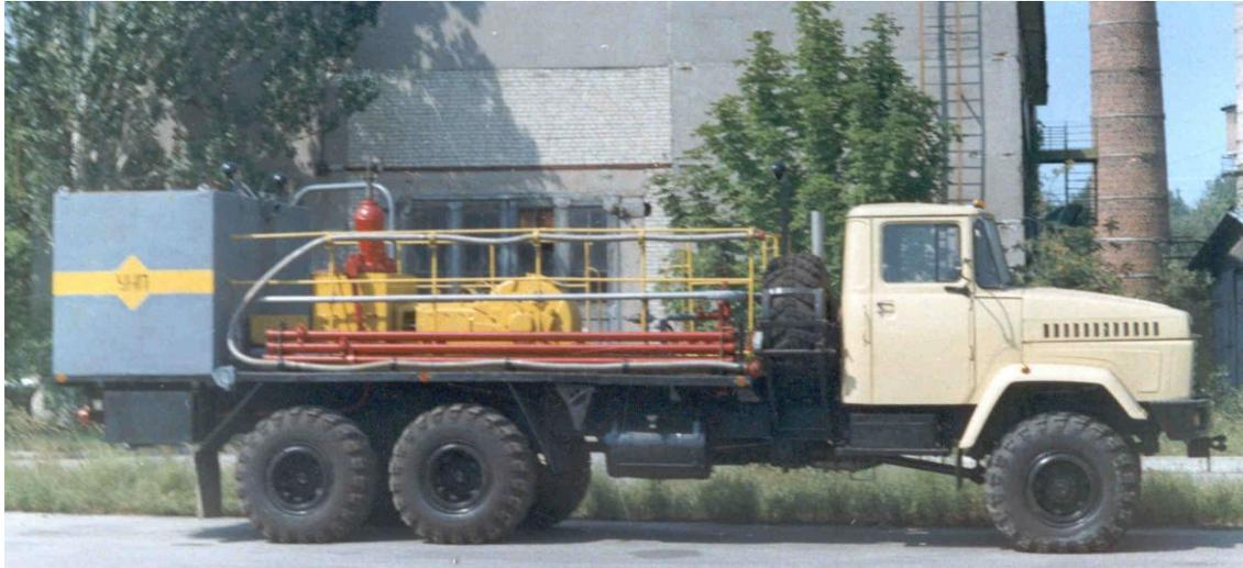
*Transportable pumping unit УНП-160x40 is used for discharging of different fluids into oil and gas wells during cementing in process of drilling and capital repair as well as during wash and driving jobs in wells.*
